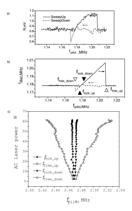
Figure 1. Experimental results for entrainment in a CW laser driven, limit-cycle, disc resonator. a) Amplitude response and b) frequency response obtained when sweeping the frequency of inertial drive. c) Entrainment region obtained when sweeping the modulation frequency of the incident laser about  $2\omega$  with no inertial drive. From [2].
