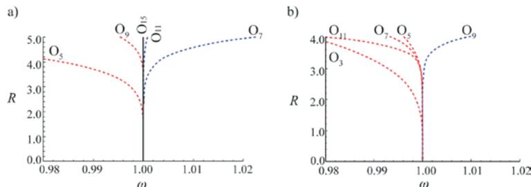
Figure 1. Backbone curves of: a) oscillator (3a); b) oscillator (2), (4a-c) rescaled with  $x \rightarrow \varepsilon x$ ,  $\varepsilon = 0.1$  for  $a_0 = 0$
