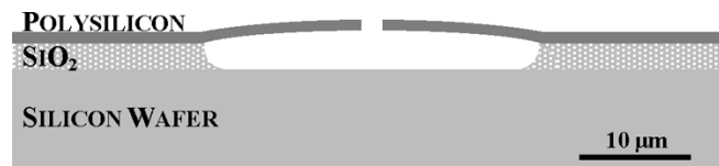
Fig. 1. Bisection of the polysilicon shell-type micromechanical resonator.
