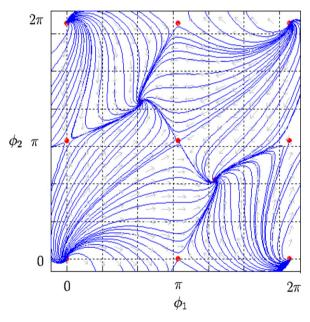
Fig. 4. Phase portrait for Eqs. (24) and (25) with  $W_1 = W_2 = 0$ . The flow has one source, three saddles and two sinks.
