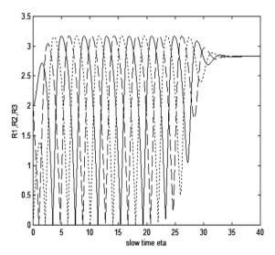
Fig. 8. Numerical integration of slow flow of Eqs. (67)–(72) for initial conditions  $a_1 = 2$ ,  $b_1 = 0.001$ ,  $a_2 = 2$ ,  $b_2 = 0.001$ ,  $a_3 = 0.001$ ,  $b_3 = 0$ . The trajectory comes close to an unstable periodic motion which is the basin boundary between the two stable steady states (64) and (65), but eventually approaches a stable equilibrium. Solid line  $= R_1$ , dashed line  $= R_2$ , and dotted line  $= R_3$ .
