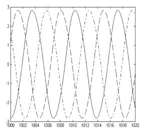
Fig. 10. Results of numerical integration of three van der Pol oscillators, Eqs. (38)–(40) for initial displacements x(0) = 3, y(0) = 1, z(0) = 2, with zero initial velocities. Time on horizontal axis omits t from 0 to 1000 to achieve steady state. Solid line = x, dot-dashed line = y, dashed line = z. Note that maxima occur in the order x, y, z, which represents a clockwise wave around Fig. 1.
