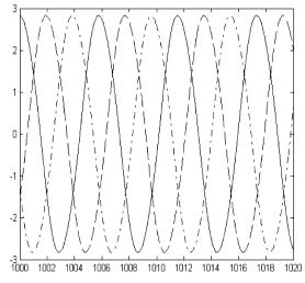
Fig. 11. Results of numerical integration of three van der Pol oscillators, Eqs. (38)–(40) for initial displacements x(0) = 3, y(0) = 2, z(0) = 1, with zero initial velocities. Time on horizontal axis omits t from 0 to 1000 to achieve steady state. Solid line = x, dot-dashed line = y, dashed line = z. Note that maxima occur in the order x, z, y, which represents a counterclockwise wave around Fig. 1.
