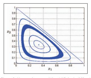
**Figure 2.** Motions of equations (14) and (15) for A = 0.02 and  $\omega = 1$  obtained by numerical integration. Here, the periodic motions of Fig. 1 are replaced by quasiperiodic motions. Note that motions starting near the equilibrium point (1/3,1/3) remain near it.
