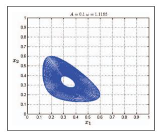
**Figure 8.** Motion of equations (14) and (15) for A = 0.1 and  $\omega = \frac{2}{\sqrt{3}} - (\frac{1}{3\sqrt{3}} + 0.2)A = 1.1155$  for initial conditions  $x_1 = x_2 = 0.3$  obtained by numerical integration. This system lies to the left of the resonance tongue in Figure 4. Note that here a motion which starts near the equilibrium (1/3,1/3) travels far away from it.
