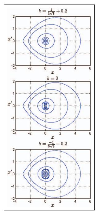
**Figure 6.** Poincare map obtained by numerically integrating equation (30) for  $\epsilon = 0.1$  and  $\omega = 2/\sqrt{3} + k\epsilon^2$ . Cf. Figure 5.
